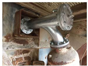
The Rapid Change Nozzle can be changed from the outside in a very short time without access to the duct/furnace/kiln/hopper.
